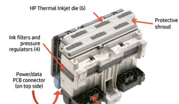
Figure 1. Printhead module used in HP PageWide large-format printers
